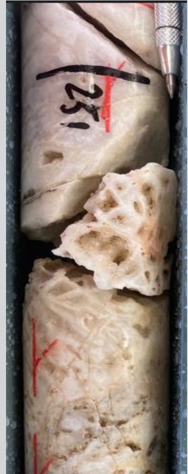
Bladed quartz after carbonate (epithermal boiling zone texture), PLRD0060, Powerline.
