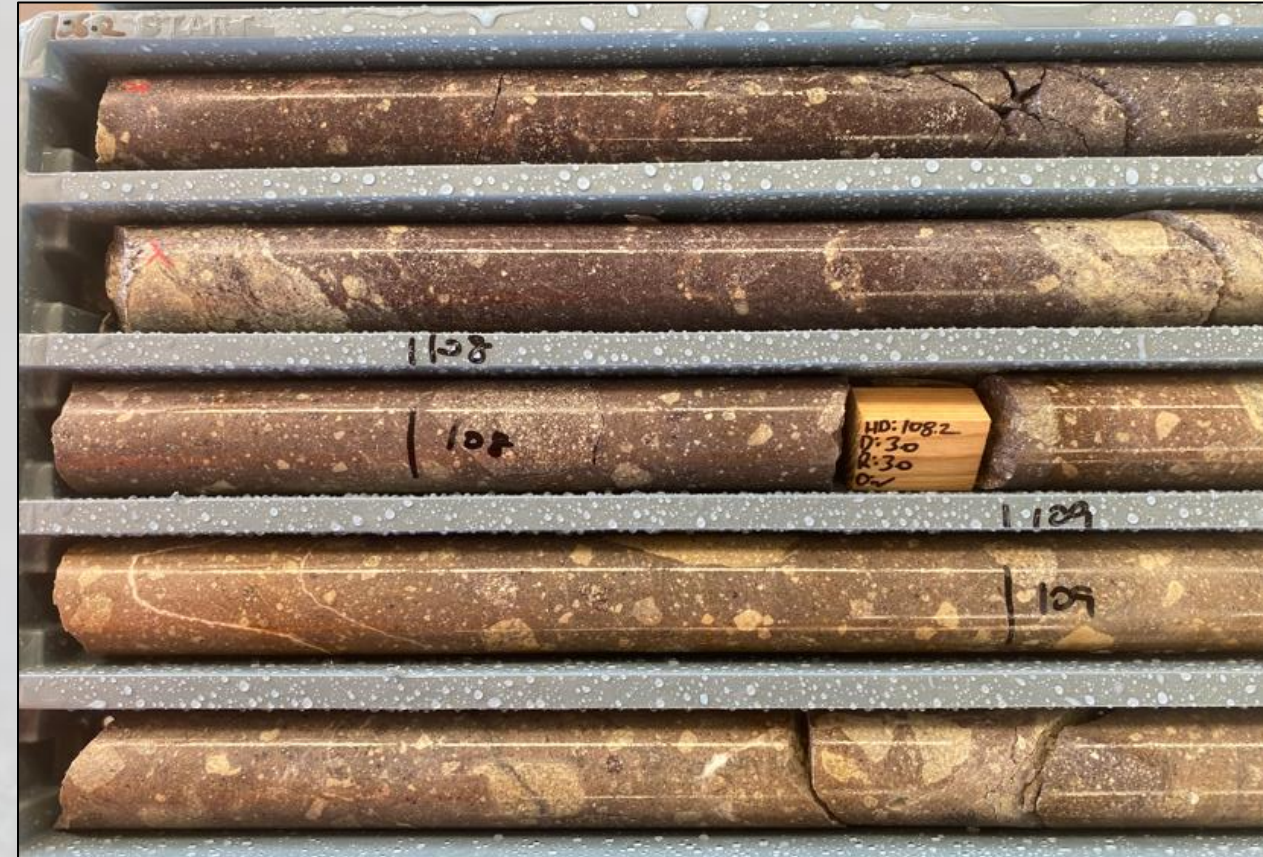
Mt Janet Andesite – Polymictic (mixed basement and volcanic derived) matrix supported pebble – cobble grade sedimentary breccia, 0775-02-VO, Voyager Deposit
