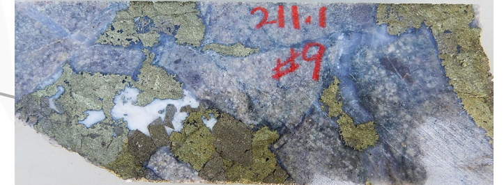
Hydrothermal breccia in which elongate and aligned clasts of sericite altered siltstone and lesser plagioclase porphyry are cemented by pyrite-chalcocopyrite, calcite and lesser quartz. Shingle-type breccia textures are indicative of decompressive shock related to sudden fluid withdrawal. 22CAEDD010, 272m.
