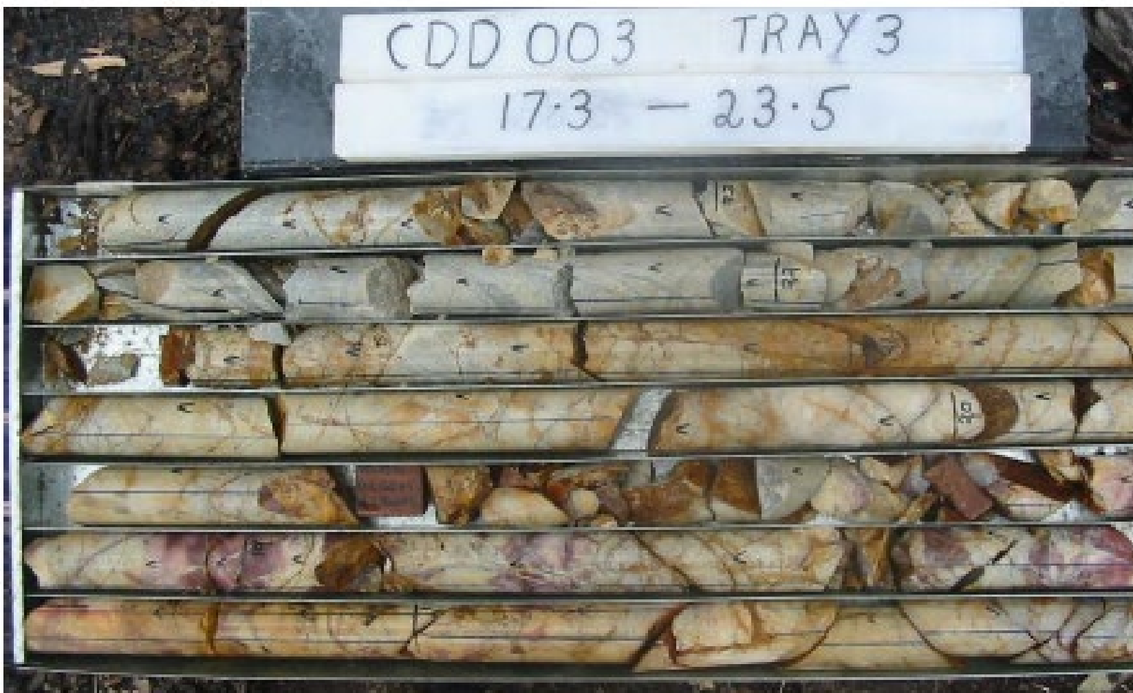
Figure 3 : Supergene Enriched Copper Zone in Partially Oxidised Rock
