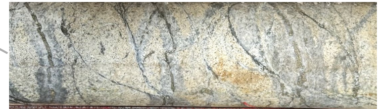
Porphyry style "D" vein pyrite sericite stockwork
