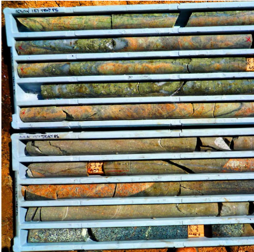
Sheeted translucent quartz veins, multiphase intrusive aplite dyke with wispy A veins, pegmatite
