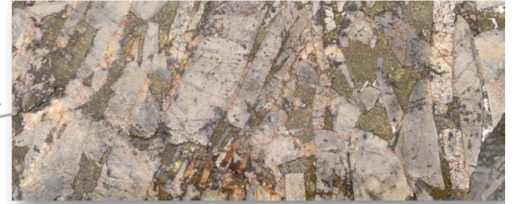
Hydrothermal breccia in which elongate and aligned clasts of sericite altered siltstone and lesser plagioclase porphyry are cemented by pyrite-chalcocopyrite, calcite and lesser quartz. Shingle-type breccia textures are indicative of decompressive shock related to sudden fluid withdrawal. 22CAEDD010, 272m.
