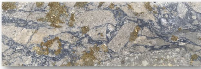
Hydrothermal breccia comprising angular to subangular clasts of sedimentary wallrock and two phases of porphyry intrusion cemented by a fine grained mix of quartz and molybdenite with lesser calcite and pyrite. Late infill by coarse grained pyrite is also present. 23CAEDD018, 346m.
