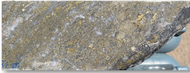
Weakly banded vein of pyrite – quartz – chalcocopyrite – tetrahedrite (black mineral, RHS of photo). 23CAEDD018, 360m.
